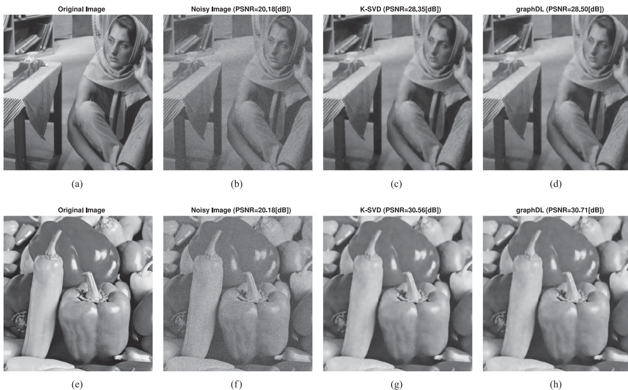
Fig. 8. Image denoising results for the images barbara and peppers: (a), (e) Original image, (b), (f) Noisy image, (c), (g) K-SVD denoising, (d), (h) graphDL denoising with optimized L .
